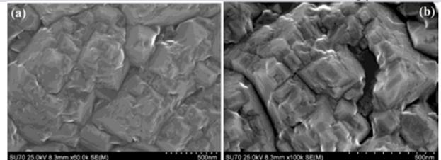
High-resolution SEM images of the nanocrystalline diamond coatings grown by chemical vapour deposition.
