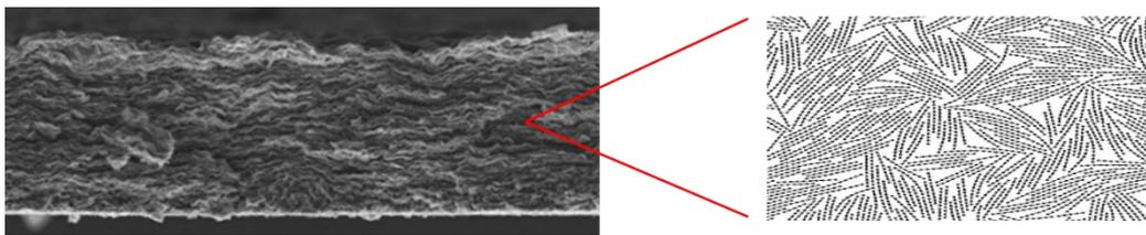
Figure: (left) Example of clay film of thickness around  $50\mu\text{m}$  and (right) example of coarse-grained molecular model.
